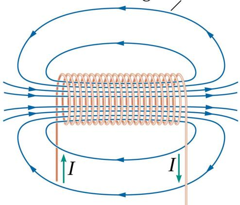
A solenoid with current running through it will create a magnetic field around it. Due to the shape of the solenoid, the field will resemble that of a bar magnet, with each end of the solenoid being the opposite poles.
